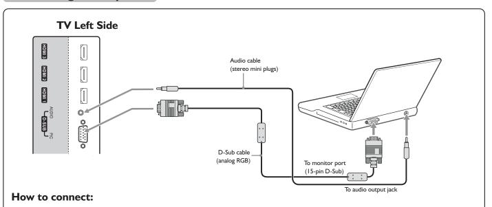
Connect a D-Sub cable between the D-SUB jack on the computer and the D-SUB input jack on the unit.
